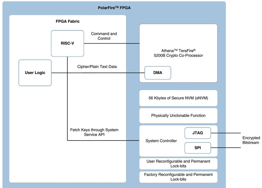
Users instantiate a RISC-V CPU for command and control, including fetching keys from the system controller through a system service API, initializing the Athena Core, and setting up DMA to perform the desired function. The TeraFire core comes with a complete firmware driver library for all supported protocols. These driver libraries are delivered to the designer's desktop through our Firmware Catalog within Libero SoC PolarFire.
