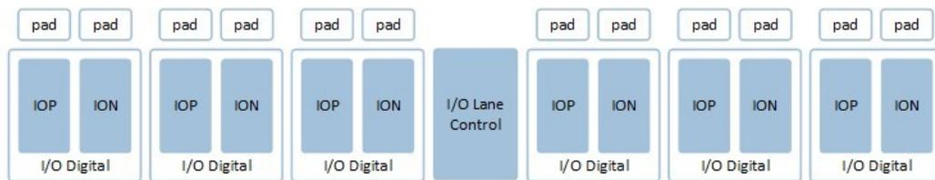
The number of I/O pins varies depending on the device and package size. The persistent I/O feature preserves a state on an I/O without user intervention during programming mode. The PolarFire FPGA I/O buffers are constructed from the following main sub modules.
